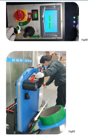
7.Then pull/push the joystick in the backwards direction until the chainlance is fully retracted into the machine
