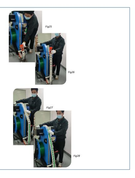
11) Remove the strap from the clamp in the chainlance and hold it straight up as shown.
