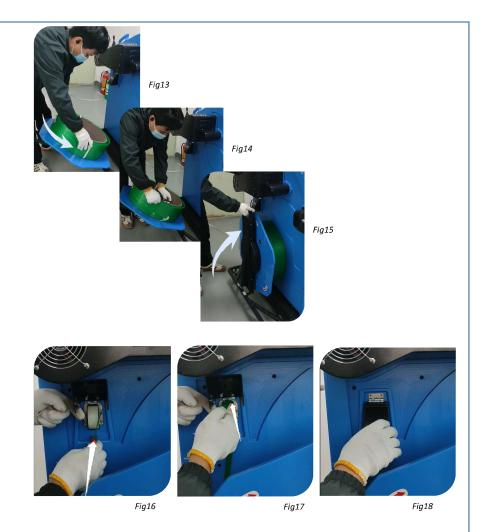
7) Open the sliding window, press the clamp lock inside the chainlance with your left hand . And then thread the strap from the right to the left through the slot in the clamp lock.
