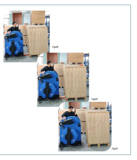
7.The strap lift arm comes up automatically after the reversing sledge moves back into the machine.At the same time,you have to let the strap slide through your left hand,otherwise, the strap lift arm will not be able to rise.
