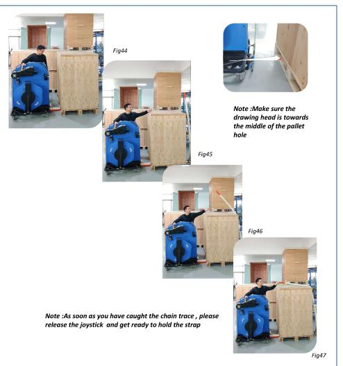
6.Hold the front of strap with the left hand as shown , move the chainlance completely backwards by pulling the joystick backwards in the " move-in " direction with the right hand .
