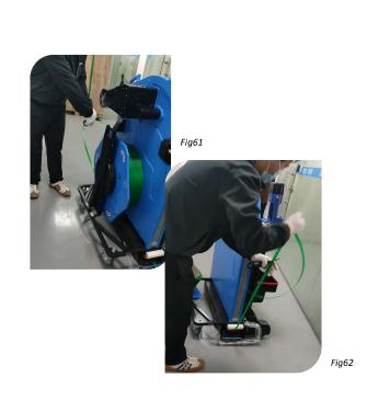
3.Set the pallet width parameter at its max 2.0meter.
