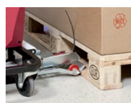
Roll the ErgoPack in front of the pallet. The chain lance...
