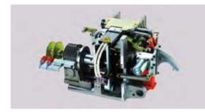
Reliable and Robust Strapping Head Robust mechanism design and high engineering standard ensure excellent durability of the machine. Use two proximity switches to replace conventional limit switches.
