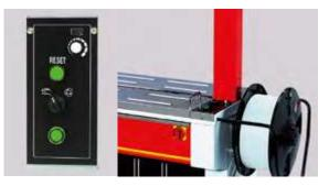
Electronic Tension Control Strap tension can be adjusted accurately by a simple turn of the dial. Easy operation.
